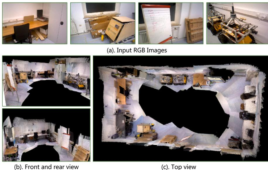
**Fig. 7.** Static point cloud reconstruction on Bonn dataset using our algorithm. (a) Input images from the dataset. (b) Front and rear views of the reconstructed point cloud. (c) Top view of the reconstructed point cloud, showcasing the spatial layout of the scene.
