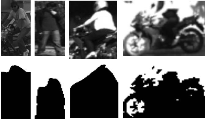
Fig. 9. Clustering results for small traffic participants on KITTI odometry outdoor driving sequences 00–10, including pedestrian, cyclist, and motorcycle-size object boxes from the same outdoor driving split. The first row is the grayscale image of the object detection box, and the second row is the foreground-background clustering result from grayscale and neural-depth cues. Black denotes foreground dynamic candidates, and white denotes retained background.
